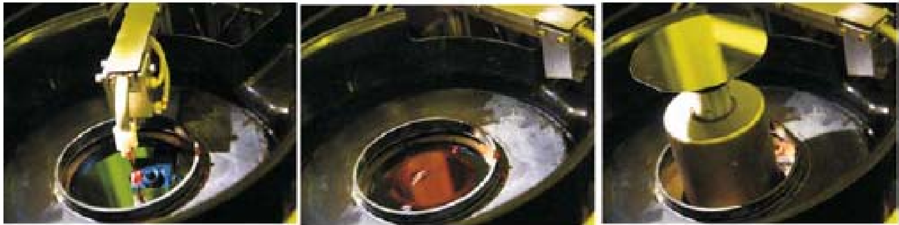
Fig. 1.37 Photoresist is roughly spilled in the middle of the wafer, centrifugal forces, during fast rotation, homogeneously distributes the resist on the wafer. Courtesy of ITE Warsaw [156]
